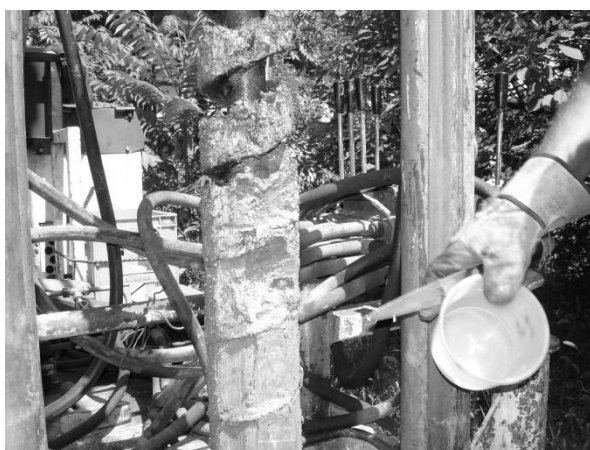
Fig.6 Prelevare probe sol tulburate
